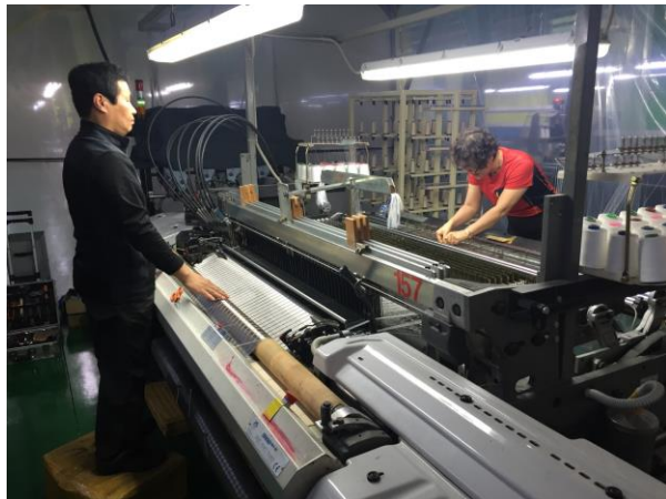
Rapier Loom of the type used for SolFab™ manufacture
